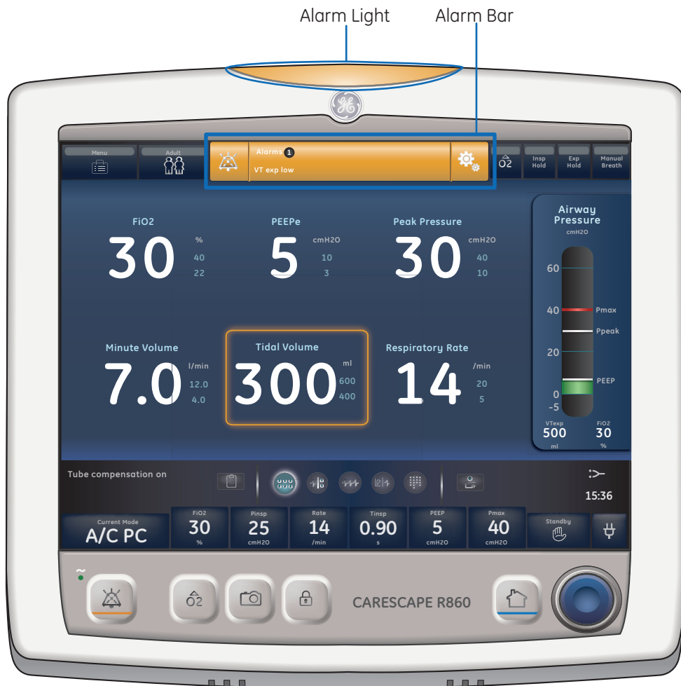
Figure 5.1 Alarm Light and Alarm Bar
